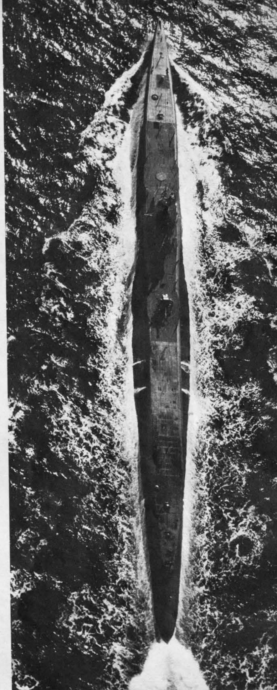
Submarine has narrowest plan of all, being built for undersea operation. Deck is slim and pointed; while hull appears to bulge abaft conning tower.
